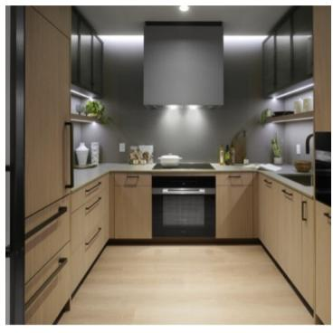
In the kitchen, a ventless range hood and charcoal filter eliminate the need for exterior venting. Photo by Tridel.
